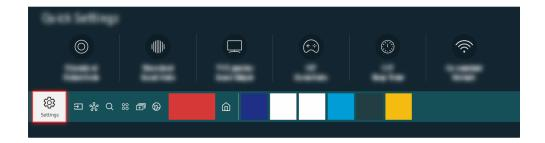
Check the volume on the screen. If a number for the TV volume is not displayed, select > Settings > Sound > Sound Output. Then, select TV Speaker.
