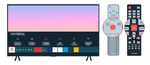
If the same problem persists, run a diagnostic test. On the remote control, press the low button. Select low > low Settings > Support > Device Care > Self Diagnosis > Picture Test.
