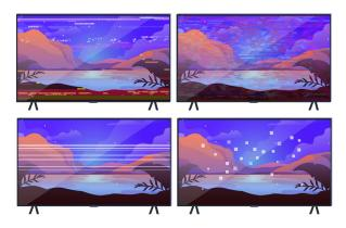
If the issue persists, define exactly what is wrong with the display. For example, mosaics and blocks, multiple lines or white dots or fixed horizontal or vertical lines.
