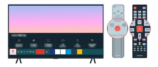
If the problem disappears during the test, check your TV signal. On the remote control, press the low button. Select low > low Settings > Support > Device Care > Self Diagnosis > Signal Information to check the signal strength.
