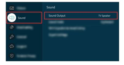
Check the volume on the screen. If a number for the TV volume is not displayed, select (a) > (b) Settings > Sound > Sound Output. Then, select TV Speaker.
