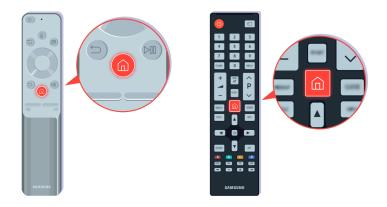
On the remote control, press the low button and move to 🕸 Settings using the directional button.
