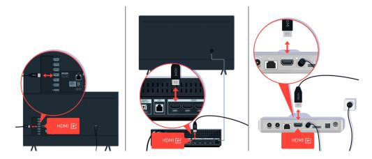
Check the antenna and HDMI cable connections.
