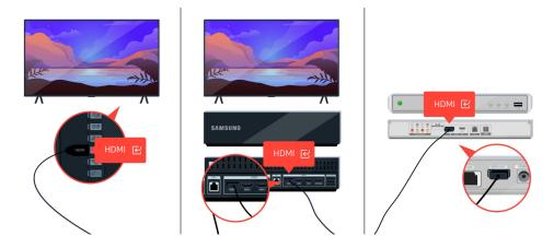
If the same problem continues, try connecting another external device to the TV using an HDMI cable. If the display is correct, your external device may be faulty.
