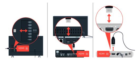
First disconnect and reconnect the power cables and HDMI cables on the back of your TV or the One Connect Box, then unplug the power cord and plug it back into the wall outlet.
