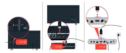
Check the antenna and HDMI cable connections.
