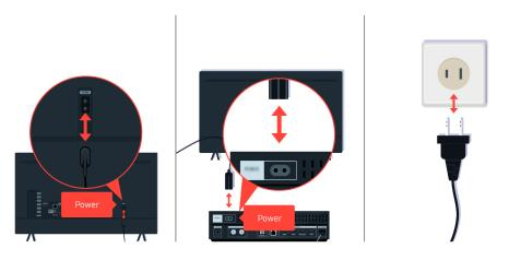
First disconnect and reconnect the power cables and HDMI cables on the back of your TV or the One Connect Box, then unplug the power cord and plug it back into the wall outlet.
