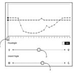
cursor (Ref. 1) at the required time on the graph, and by moving the sliders under the graph (Ref. 2, 3) define the comfortable brightness and temperature for each hour. If you want to apply the new configuration immediately, exit the graph parameters and confirm the new settings. When a configuration is pressed, a context menu will appear that will allow you to manage custom Frontlight settings:
