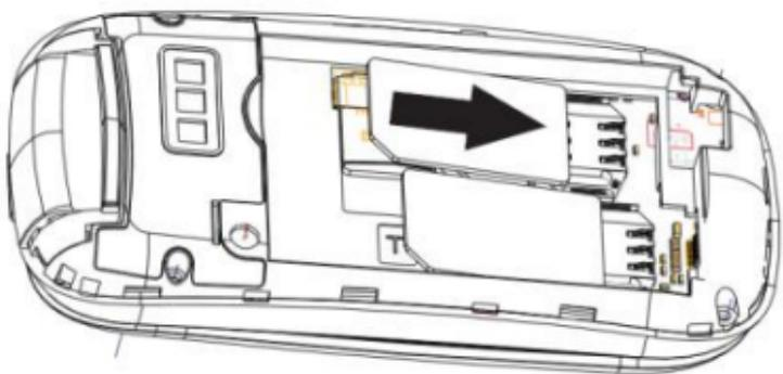
2. Take out SIM card: Hold the notch of SIM card and lift it slightly down by the other hand to take card out.
