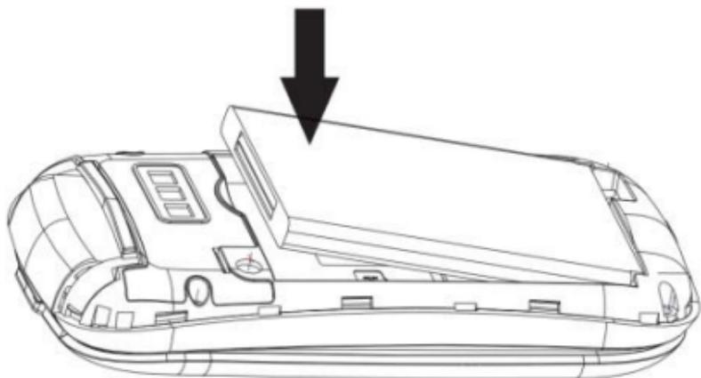
3. Close the battery cover. Make sure that cover is completely matched and the cover matching sound could be heard.
