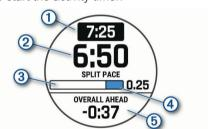
The device displays your target split pace ①, current split pace ②, completion progress for the split ③, distance remaining in the split ④, and overall time ahead or behind of your target pace ⑤.
