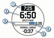
The device displays your target split pace ①, current split pace ②, completion progress for the split ③, distance remaining in the split ④, and overall time ahead or behind of your target pace ⑤.
