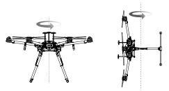
4. Recalibrate the compass if the Aircraft Status Indicator blinks red.
