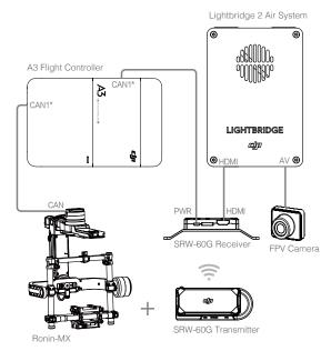
When using the Ronin-MX, set the App Output Mode in the DJI GO app to display the image on your mobile device from the camera used with the Ronin-MX. Launch the DJI GO app > Camera View > HD<sub>ull</sub> > Disable EXT Port, adjust the Bandwidth Allocation to ensure that the "HDMI" percentage is more than 0%, and then set the App Output Mode to HDMI.
