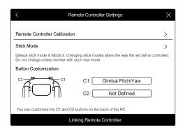
Press the C1 or C2 button to switch between pitch mode and yaw mode. Use the gimbal dial to control the tilt/pan motion of the camera.
