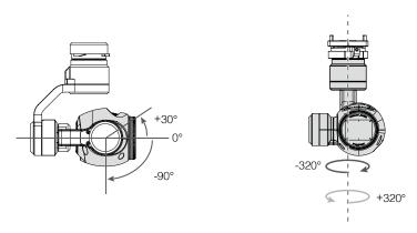
Under the default settings, turn the gimbal dial on the remote controller to tilt the camera. Note that you cannot simultaneously tilt and pan the camera in the Single Remote Controller mode. Enable the Master-and-Slave mode in the DJI GO app and set a second remote controller to Slave if you wish to tilt and pan the camera together.
