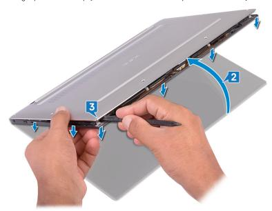
Moving the base cover from left to right, release the clips securing the base cover to the palm-rest assembly.
