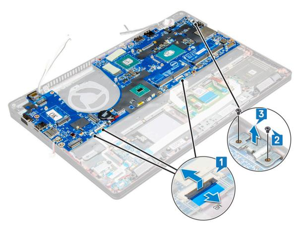
Remove the M2x3 screws (3) and lift the system board away from the computer [1, 2].
