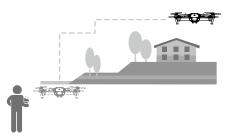
The aircraft will automatically adjust its speed when it senses an obstacle in front or if it is flying too close to the ground. However, this feature should not be relied upon for navigation between obstacles. Failsafe procedures will override TapFly. If the GPS signal weakens, the aircraft will exit autonomous flight and return to home.
