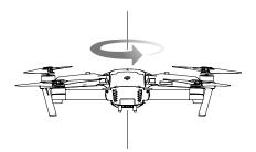
Hold the aircraft vertically, with nose pointing downward, and rotate it 360 degrees around the center axis.
