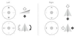
Move the aircraft upwards, downwards or rotate to the left or right by pressing on the left half of the screen. Move the aircraft forwards, backwards or rotate to the left or right by pressing on the right half of the screen.
