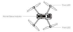
The Front LEDs show the orientation of the aircraft. The Front LEDs glow solid red when the aircraft is turned on to indicate the front (or nose) of the aircraft (the Front LED can be turned off in the DJI GO 4 app). The Aircraft Status Indicator communicates the system status of the flight controller. Refer to the table below for more information about the Aircraft Status Indicator.
