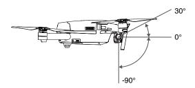
Use the gimbal dial on the remote controller to control camera tilt, or go to Camera View in the DJI GO 4 app, tap and hold on the screen until a blue circle appears, then drag the circle to control the camera's tilt.
